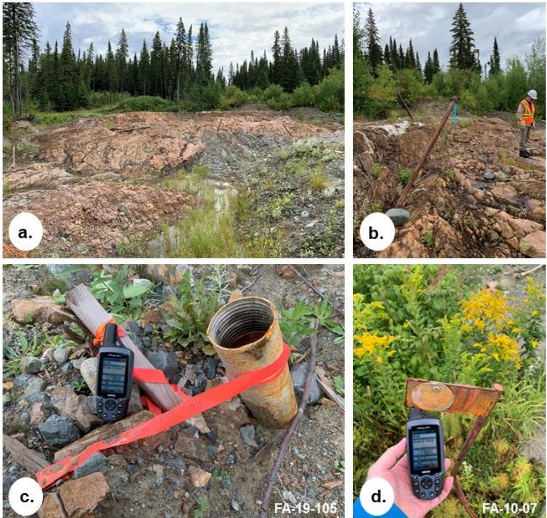
a) Fayolle main stripping (exposure of Zone 3 gold mineralization) and drilling/channel sites; b) Historical drill hole casings on the main stripping area; c) Drill hole casing from the 2019 program (FA-19-105); d) Historical drill hole casing from the 2010 program (FA-10-07).
