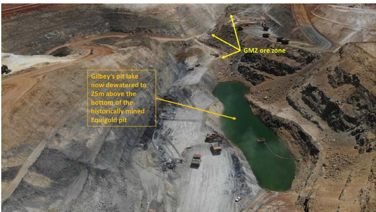
Figure 3: Gilbey's Pit Lake Now Effectively Dewatered to a Point Where There Will Be No Impact on Mining (Gilbey's pit looking south)
