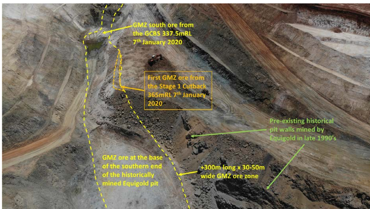
Figure 2: Showing the +300m length of GMZ ore zone now exposed in the southern end of the Gilbey's pit.
