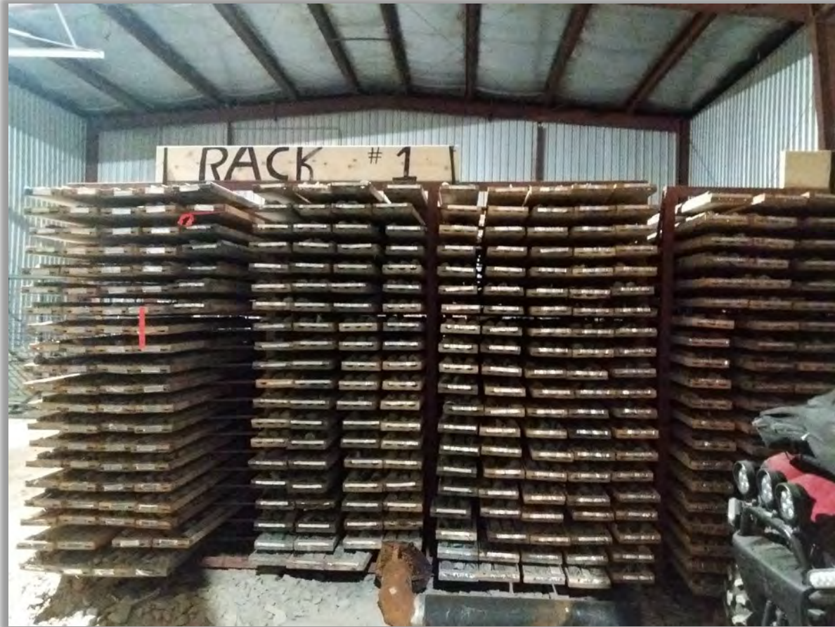
Figure 5.2 Internal Core Storage Racks on Goldboro Property
