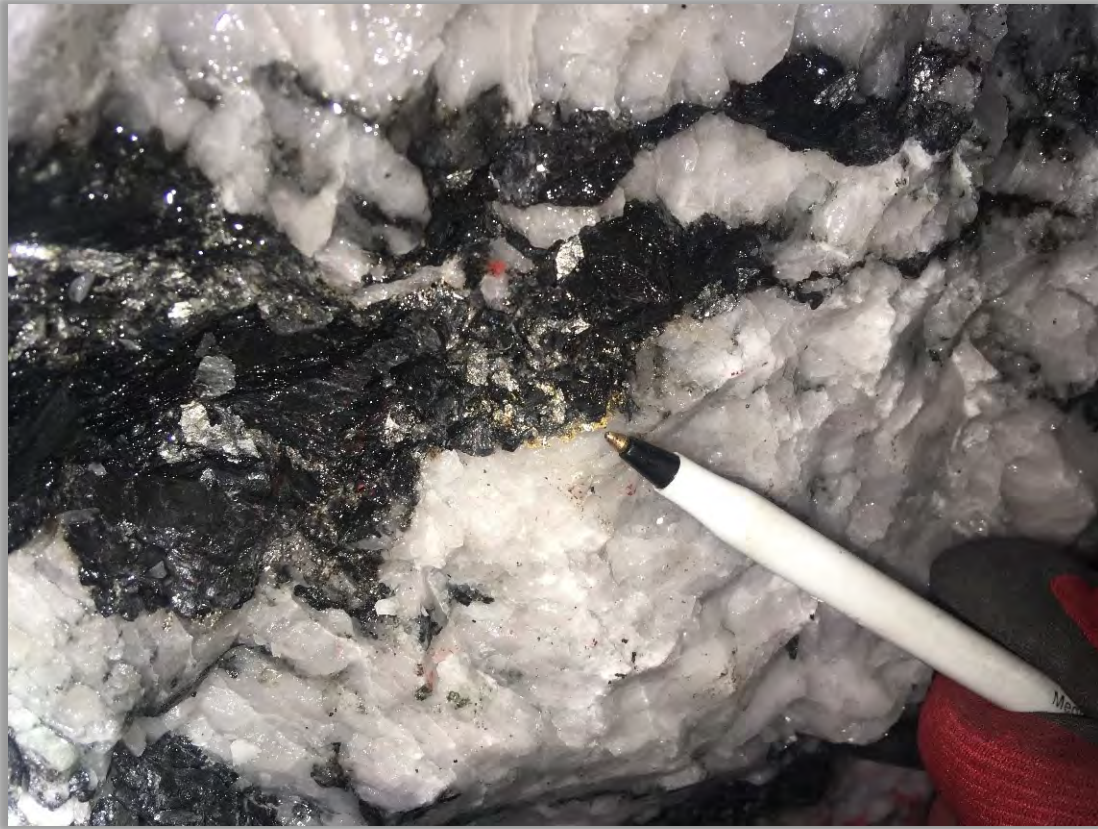
Figure 9.12 Visible Gold Along Margin of Quartz Vein- Argillite Contact in Level 3 East Round 3
