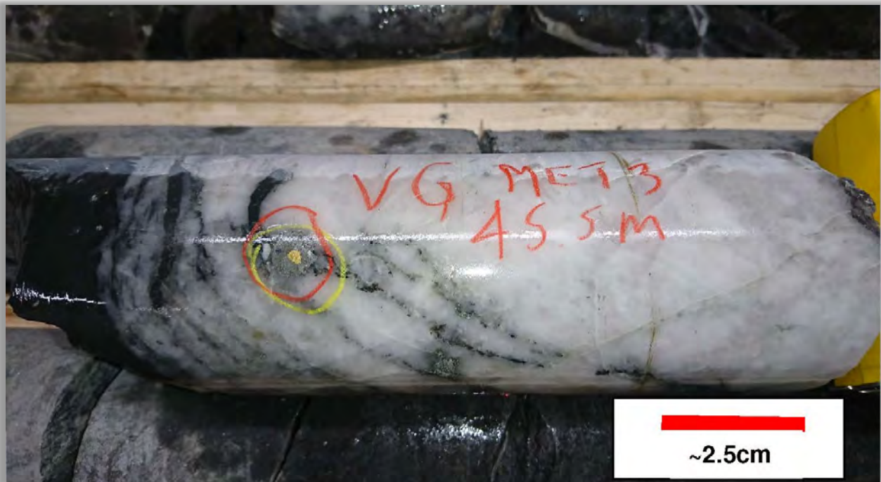
A 3 mm grain of visible gold in a crack seal, bedding parallel white quartz vein.
