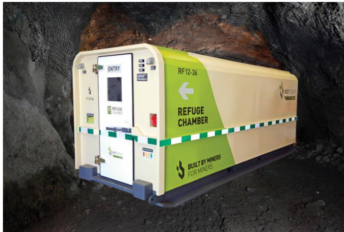
Figure 16.12 Typical Mobile Refuge Station
