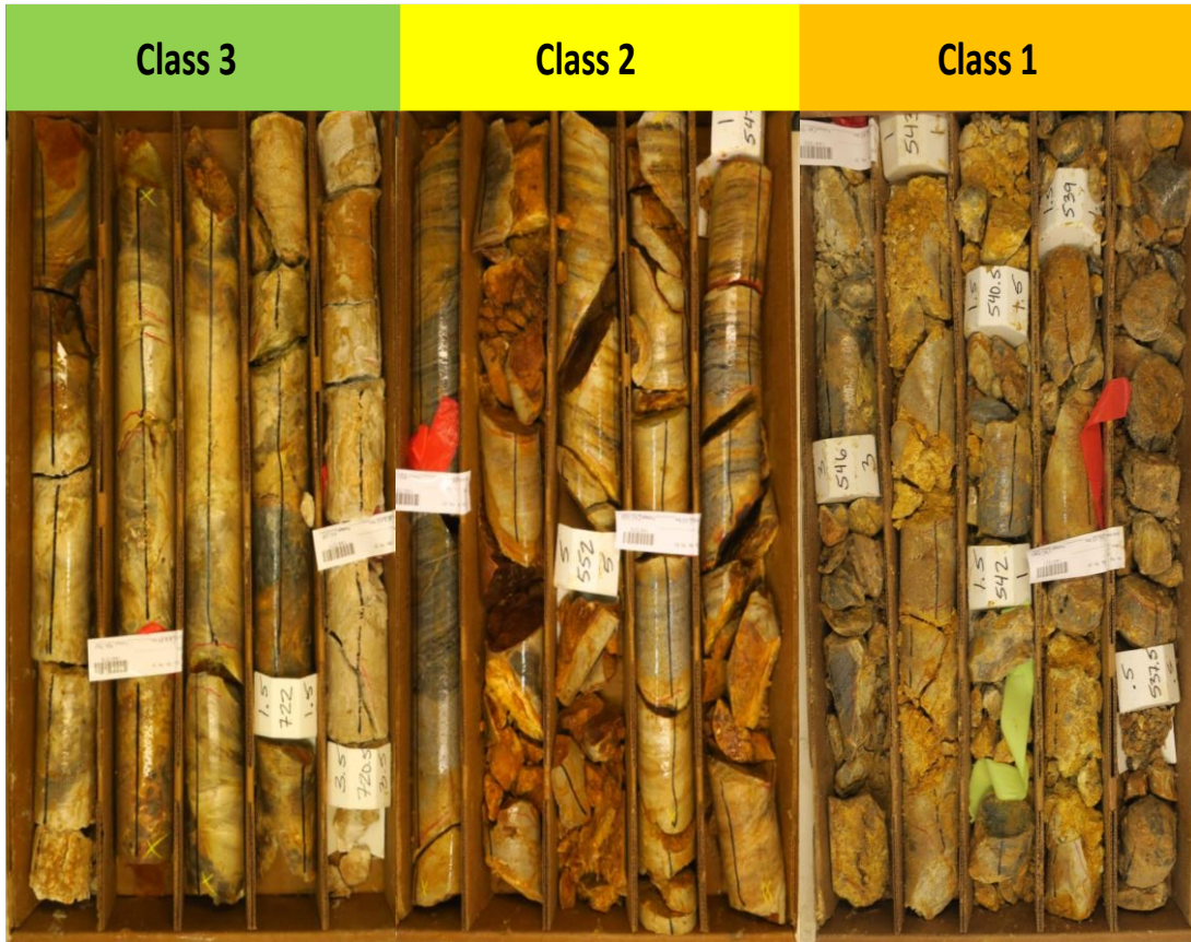
Figure 16.5 Examples of Three Geotechnical Rock Classes
