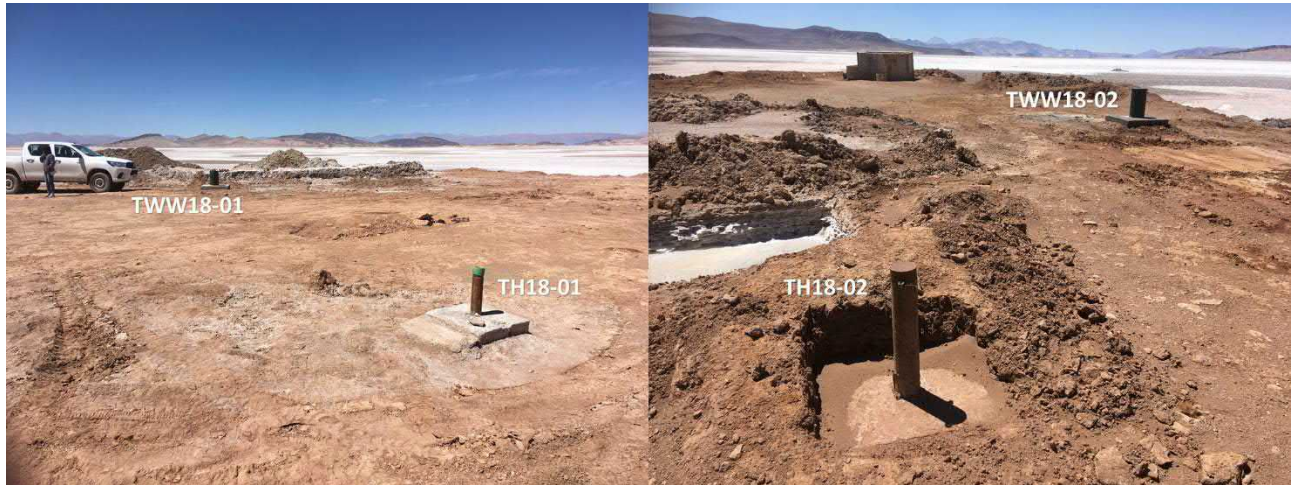
Photo 1: Two Core Holes and Two Well Holes on the Salar (Source: KP/JDS 2019)
