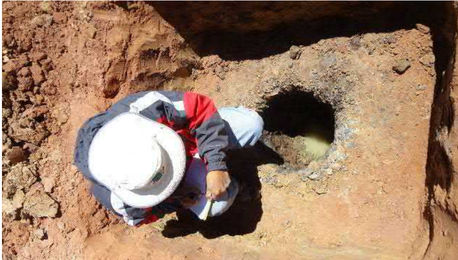
Figure 11-2: Hand-dug Pit Excavated on the Salar Surface; Note Shallow Depth to Brine
