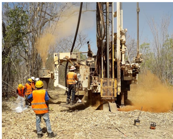
Operating RC Drill Rig
