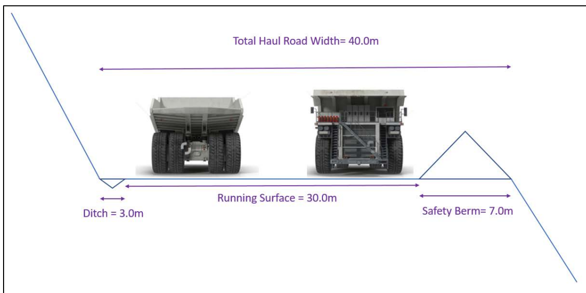
Figure 15-3: Typical haul road cross-section
