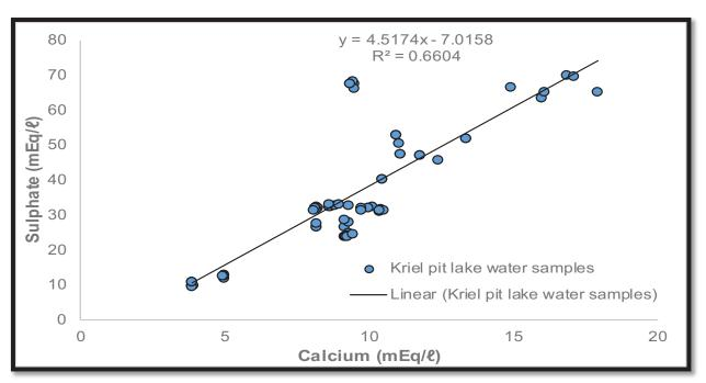
Figure 5-43: Kriel Pitlakes Ramp 44 North: Scatter plot of sulphate versus calcium.
