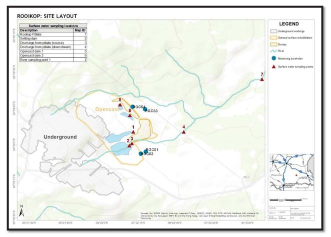
Figure 6-2: Rooikop: Mining operations and groundwater and surface water monitoring points.
