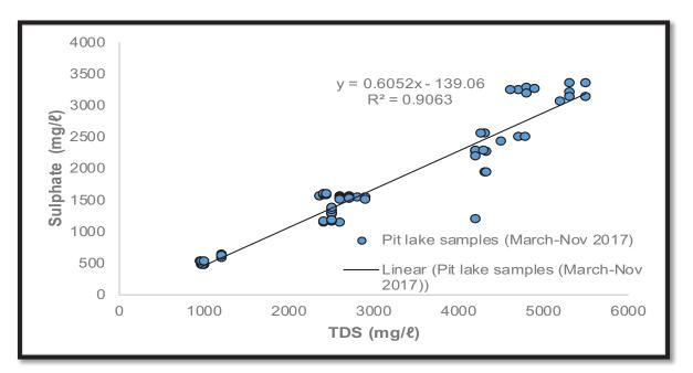
Figure 5-39: Kriel Ramp 44N, Ramp 44S and Ramp 42S: Scatter plot of TDS and sulphate
