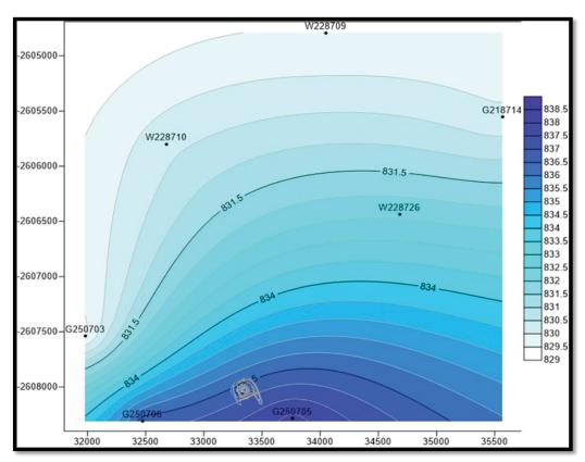
Figure 4-14: Mafutha Pitlake: Fractured aquifer groundwater flow.
