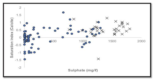
Figure 5-38: Kriel: Saturation state of sulphate in groundwater.
