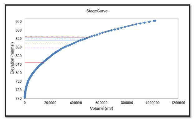
Figure 4-23 is a stage curve plot of Mafutha which demonstrates the water elevation and volume of water of the pitlake at the end of each year. The net inflow decreases as the pitlake approaches equilibrium.
