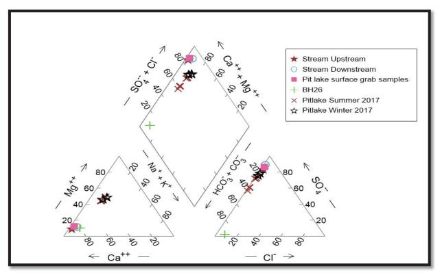
Figure 7-13: Kleinfontein Pitlakes: Piper Diagram of groundwater, surface water and pitlake.
