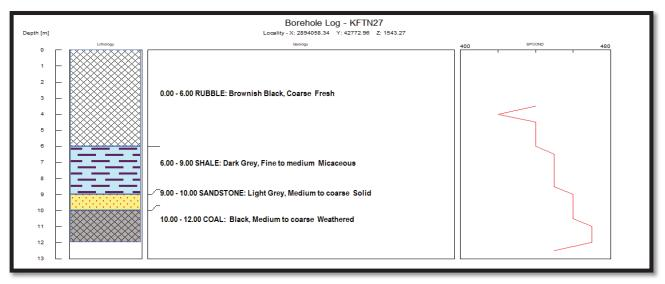
Figure 7-11: Kleinfontein Borehole KFTN27 Geology and EC profile.
