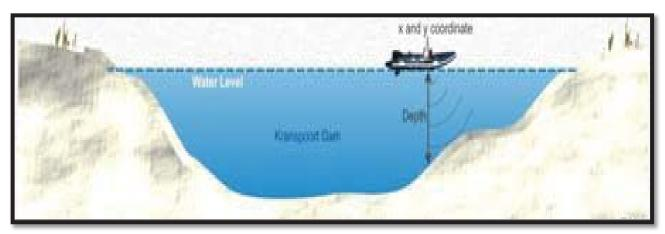
Figure 3-4: Illustration of a bathymetric survey conducted on a pitlake.
