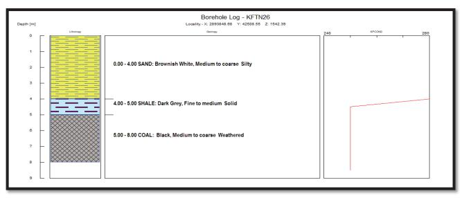
Figure 7-10: Kleinfontein Borehole KFTN 26 .Geology and EC profile
