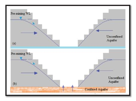
Figure 2-4: Hydrogeological conditions profiles (after Singh and Atkins, 1985)
