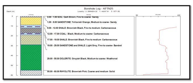
Figure 7-9: Kleinfontein Borehole KFTN25: Geology and EC profile
