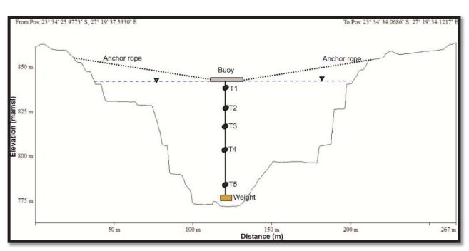
Figure 3-3: Schematic of the Mafutha pitlake temperature measuring system.
