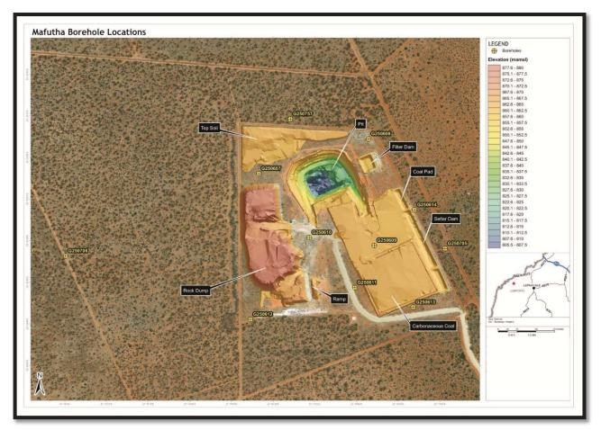
Figure 4-2: Mafutha Pitlake: Topography and location of monitoring boreholes.
