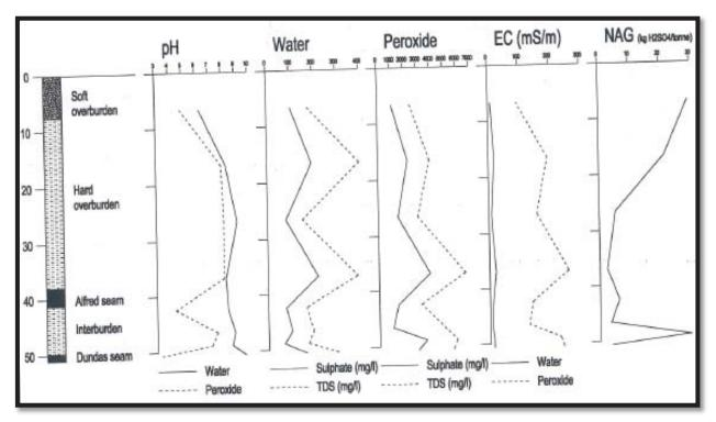
Figure 6-6: Water and Peroxide leach test results for a vertical lithological profile at Rooikop mine.
