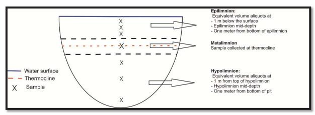
Figure 3-1: Bathtub model for pitlake sampling (Modified from Ohio EPA, 2010).
