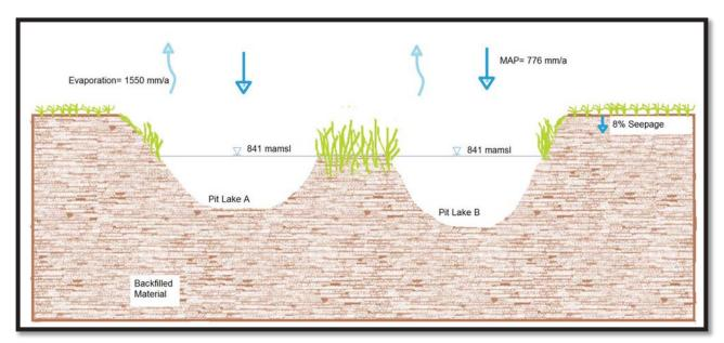
Figure 7-6: Kleinfontein Conceptual Hydrogeological Model
