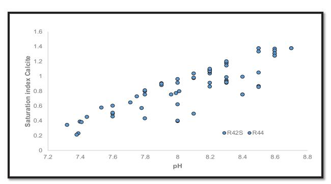
Figure 5-41: Kriel Pitlakes: Saturation index for calcite as a function of pH.
