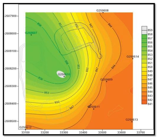
Figure 4-13: Mafutha Pitlake: Weathered aquifer piezometric levels.
