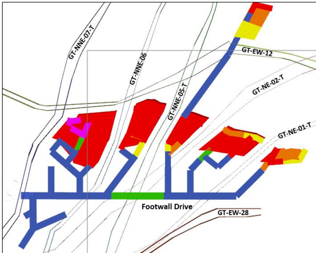
Figure 16-9: 1,225 mRL level showing main influencing faults
