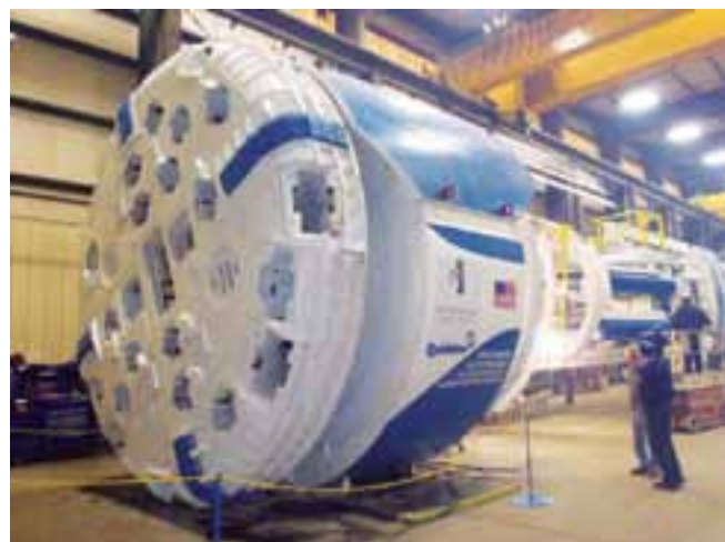
Tunnel Boring Machine (TBM) head in the launch chamber for the blitz project.
