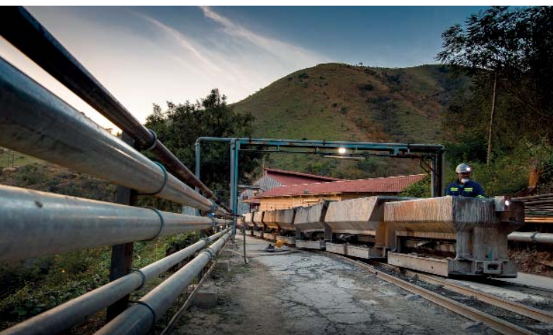
▼ Barberton Mines – hoppers carrying ore at Fairview 11 Level adit
