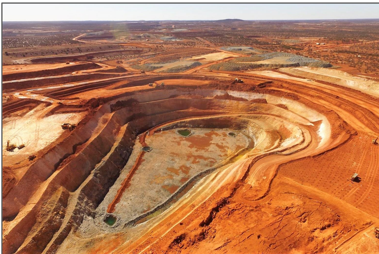
Figure 4: Eridanus pit looking North – showing cutback commencement
