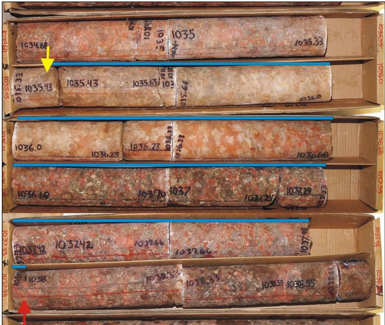
Figure 16: 82.6 mm (3¼") diameter potash core from drillhole PCS Tantalton 08-02-18-32 W1. The top of the best 2.59 m (8.5') potash interval for this drillhole is indicated by the yellow arrow at 1035.41 m depth, and the base of the interval is indicated by the red arrow at 1038.00 m. The blue line highlights the best 2.59 m potash interval.
