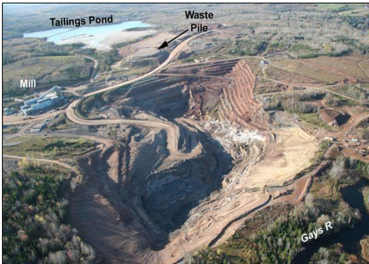
Figure 5.1: Scotia Mine Site Photo Showing the Previous Open-Pit Mine, Mill, Waste Dump and Tailings Facility (picture circa 2011)
