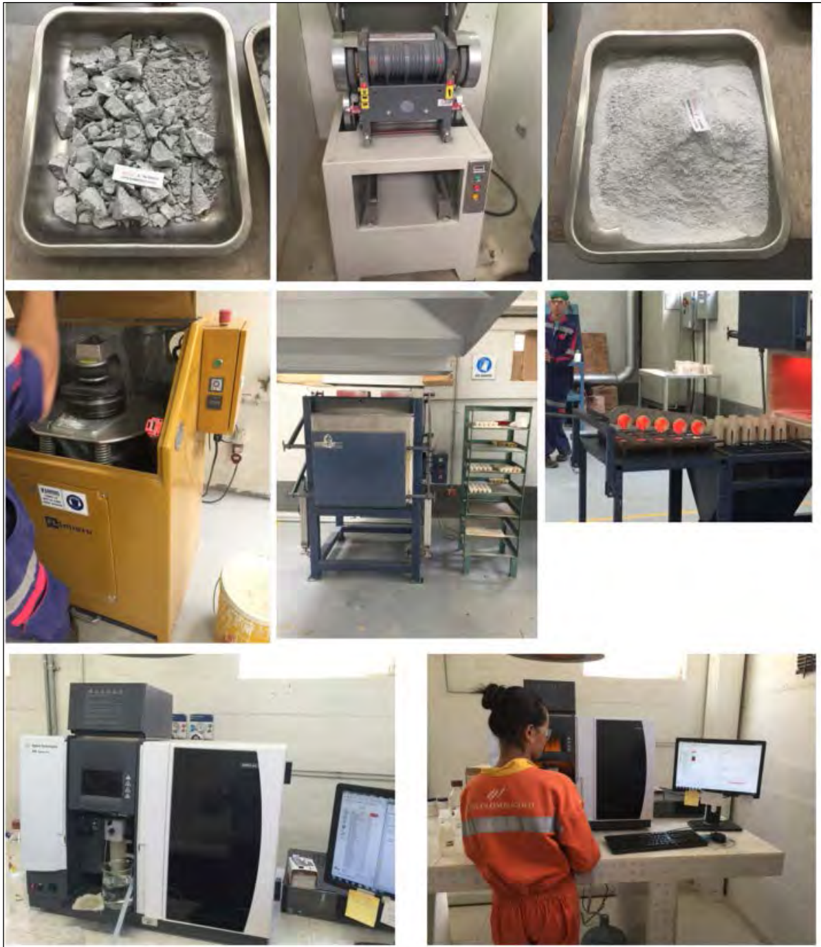
Figure 11-2: New Mine Laboratory at Segovia, Showing Crusher, Pulverizer, Furnace and AA Assay Capture
