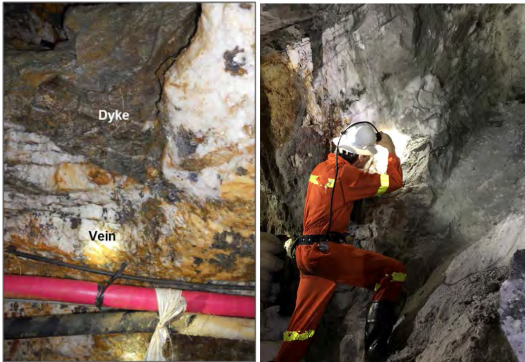
Figure 7-8: Vein Exposures in Underground Workings at El Silencio Showing Relationship with Dykes (left) and Typical Vein Thickness (right)
