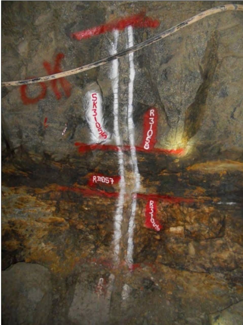
Figure 9-3: Channel Sampling Completed by Company During 2016 Sampling Program
