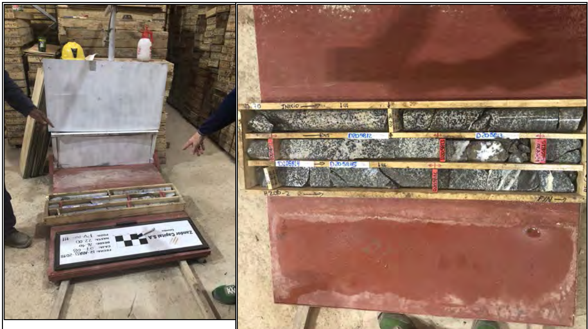
Figure 10-5: Example of Core Photography Setup (left) and Core Photographs (right)
