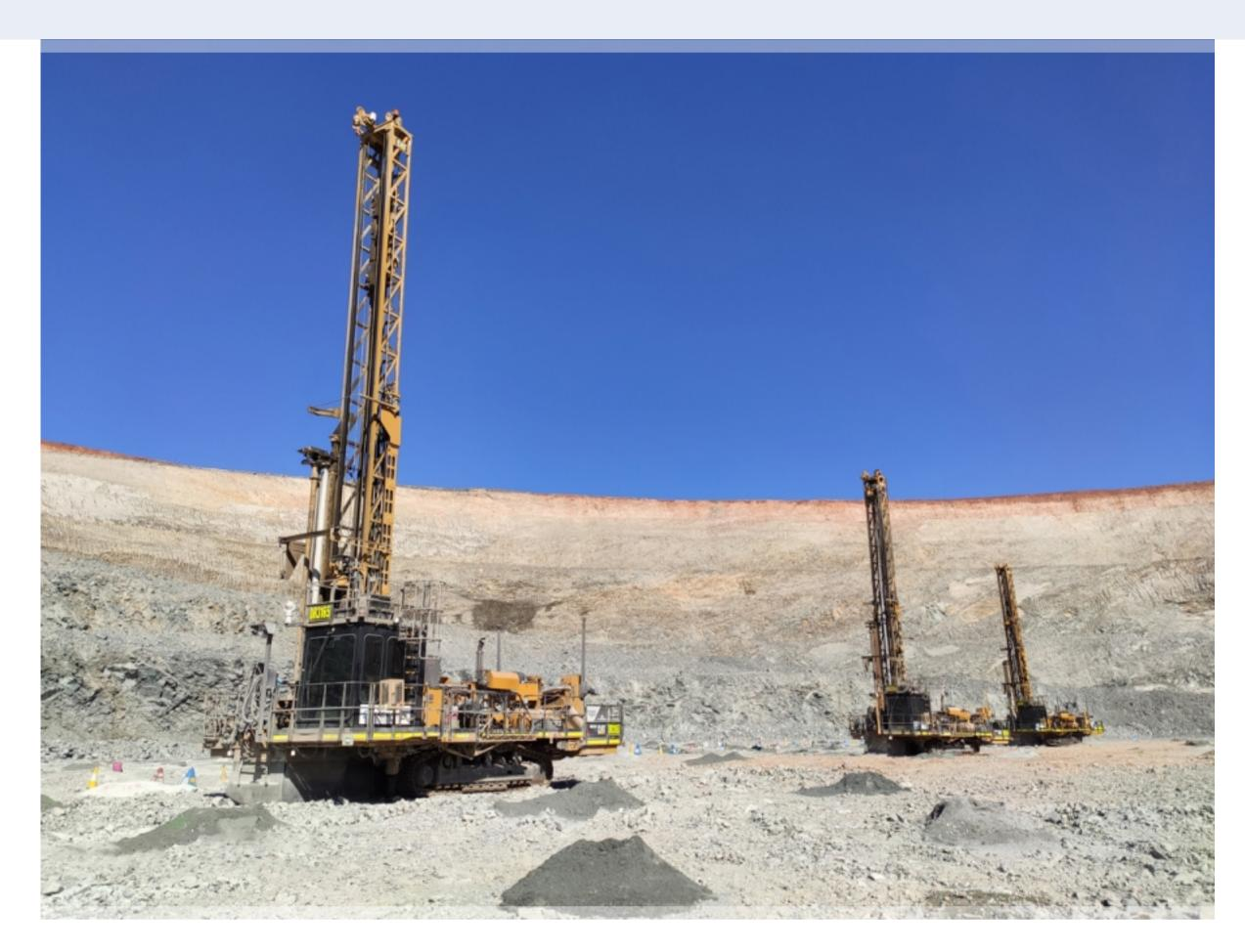
The rollout of a \$6 million autonomous drill fleet at the Tropicana Gold Mine is believed to be an industry first for hard rock mining using hammer versus the more traditional rotary concept when it comes to blast-hole drilling.
