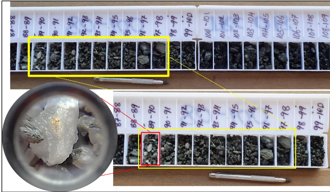
Figure 16: TRC013 visible gold and mineralised interval – record intercept 1m at 251.27g/t Au
