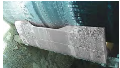
As the center of the blade wears unevenly, the outer edges create a 'smiley face' or 'mooning.'
