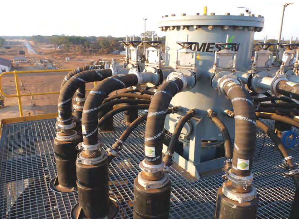
Jameson Cells, similar to the one pictured here, are credited with recovering some $30 billion in export coal in 2013 alone. (Photo: Glencore Technology)
