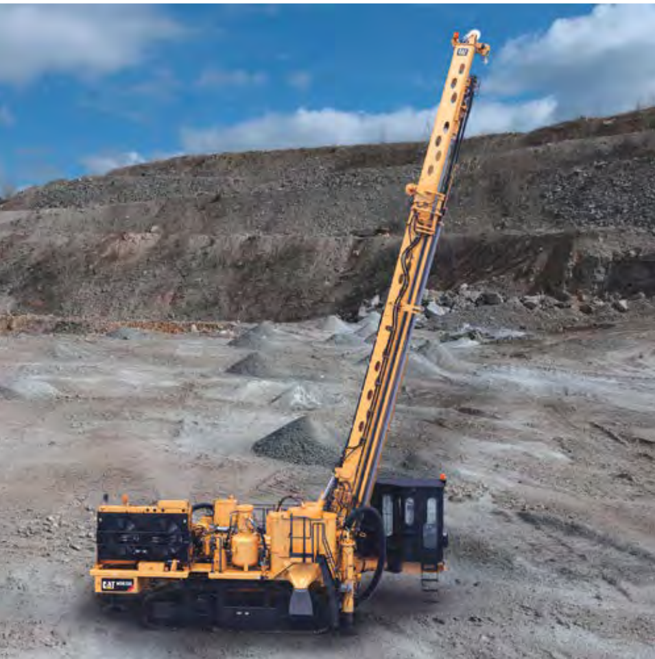
The MD6200 is the smallest model in Caterpillar's revamped line of rotary blasthole drills.
