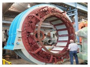
Shaft winder repairs (armature)
