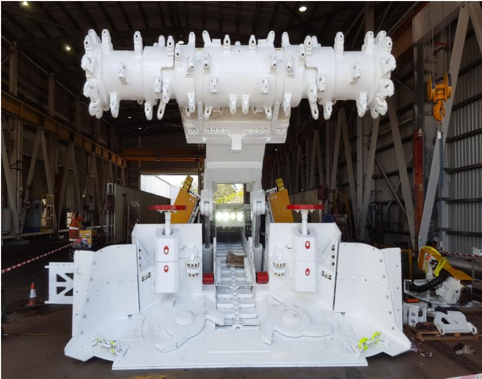
Continuous miner overhauled and underground for development mining and roadways
