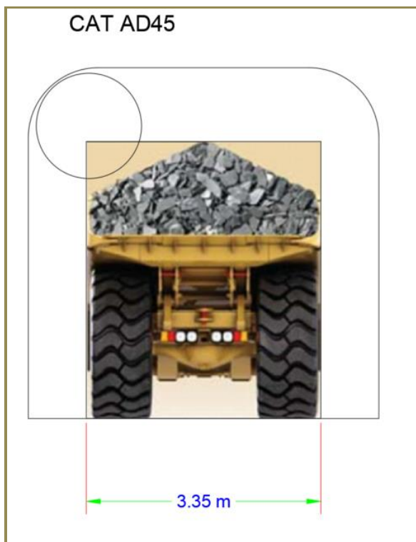
Figure 16-20: Haul Truck Clearance for Truck Size Selected
