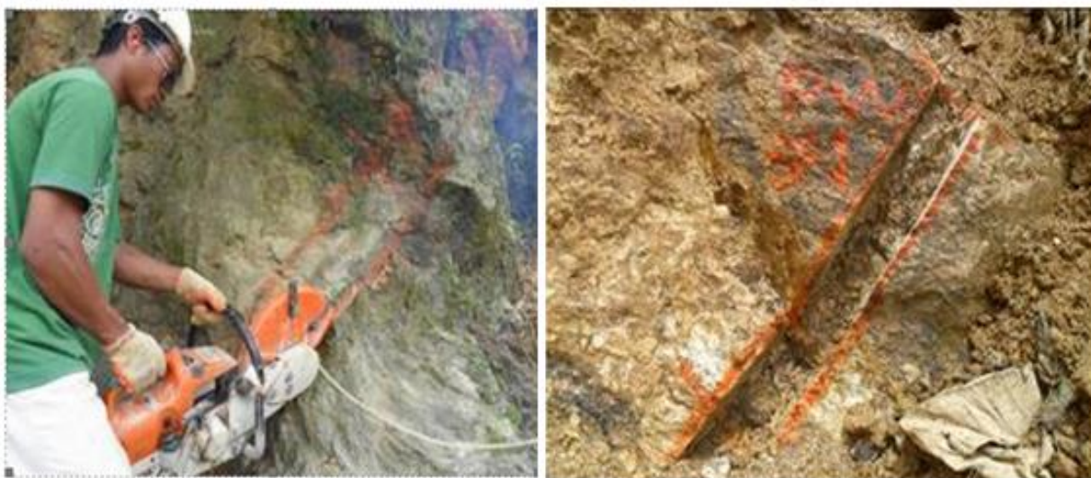
Figure 9-1: Photo of channel sampling using rock saw.
