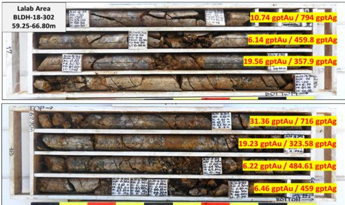
Figure 8-12: BX3 zone intercepted by drilling at Lalab area showing high Au and Ag values.
