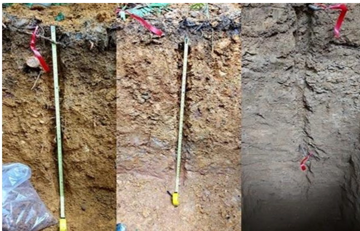
Figure 9-8: Section view of a test pit.
