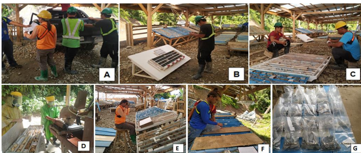
Figure 10-1: (A) Receiving of drill core samples from the drill site; (B) Core photography by a core house aide; (C) Wrapping of samples using clear packaging tape prior to cutting; (D) Core cutting by samples by designated core cutters; (E) Geologist conducting detailed core logging; (F) Sample preparation by a core house aide; (G) 25 samples with sample numbers ready for dispatch.
