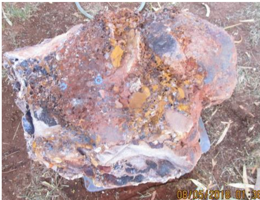
Figure 7-7. Gold particles shown within blue circles amongst buckshot pyrite (black dots) from an ferruginous channel conglomerate (South Hill).
