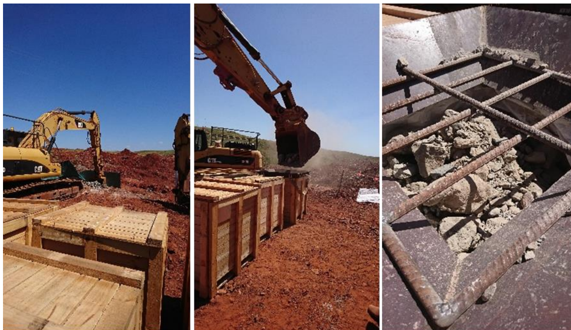
Figure 13-2. Wooden crates and metal hopper with grizzly.
