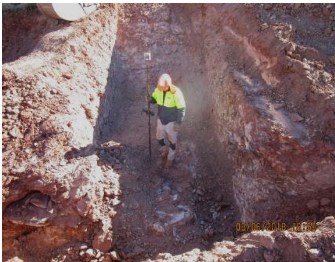
Figure 9-1. Measuring trench bulk sample.
