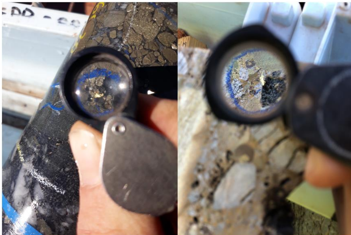
Figure 7-8. Gold in drill core. Left: BCDD18-002, 60.8-61.3m, 7.3 g/t Au. Right, BCDD18-001, 6.12-6.6 m, 4.3 g/t Au.
