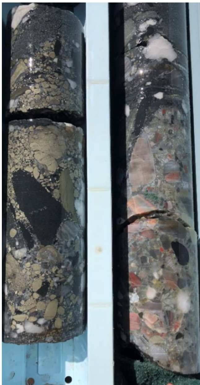
Figure 7-13. Detrital pyrite and dromedary boulder (bottom right) in 2018 PQ drill fresh mineralized core (85 mm diameter).
