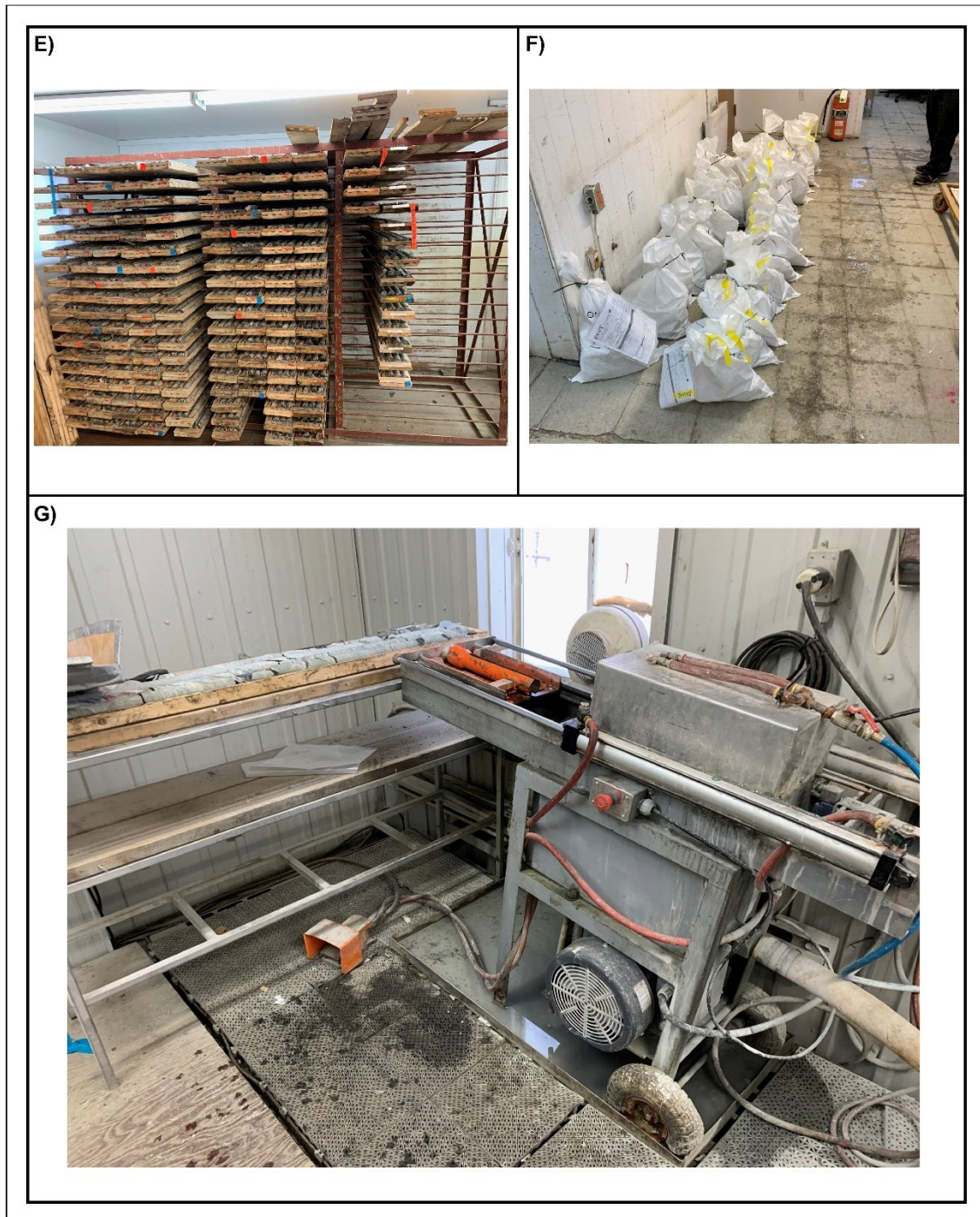
E) Interior storage ready to be sampled; F) Samples shipment with work order for the laboratory; G) Core cutting installation (Pelletier, 2020)
