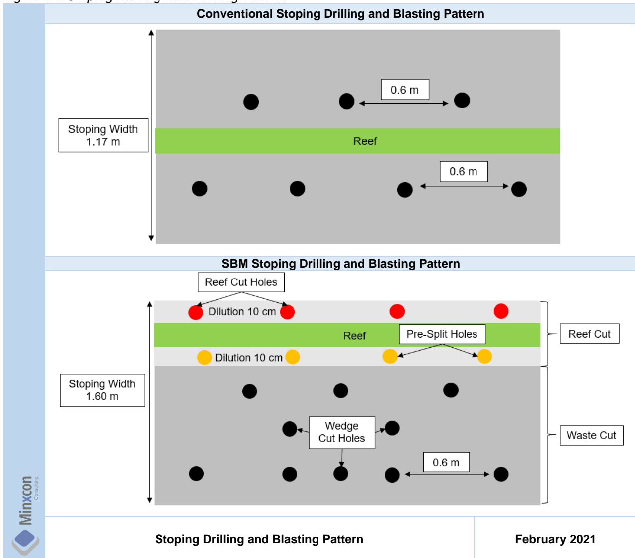
Figure 84: Stoping Drilling and Blasting Pattern
