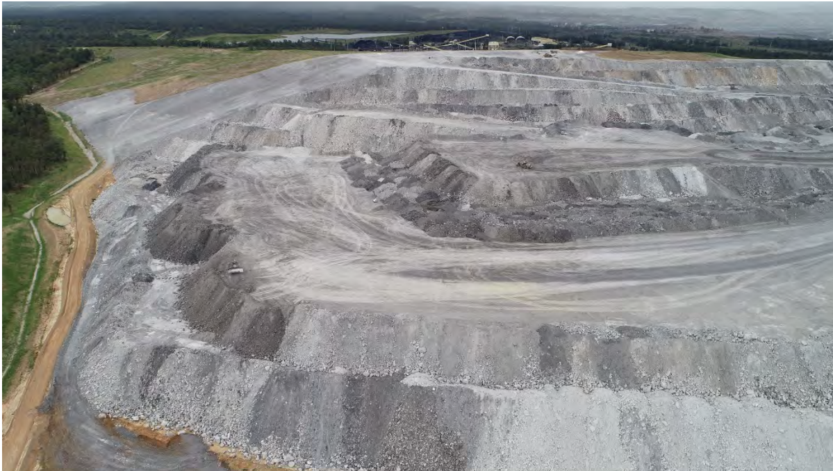
Photo 7 Dump design surface, showing the shape of ridges and drainage lines dumped out for each bench.
