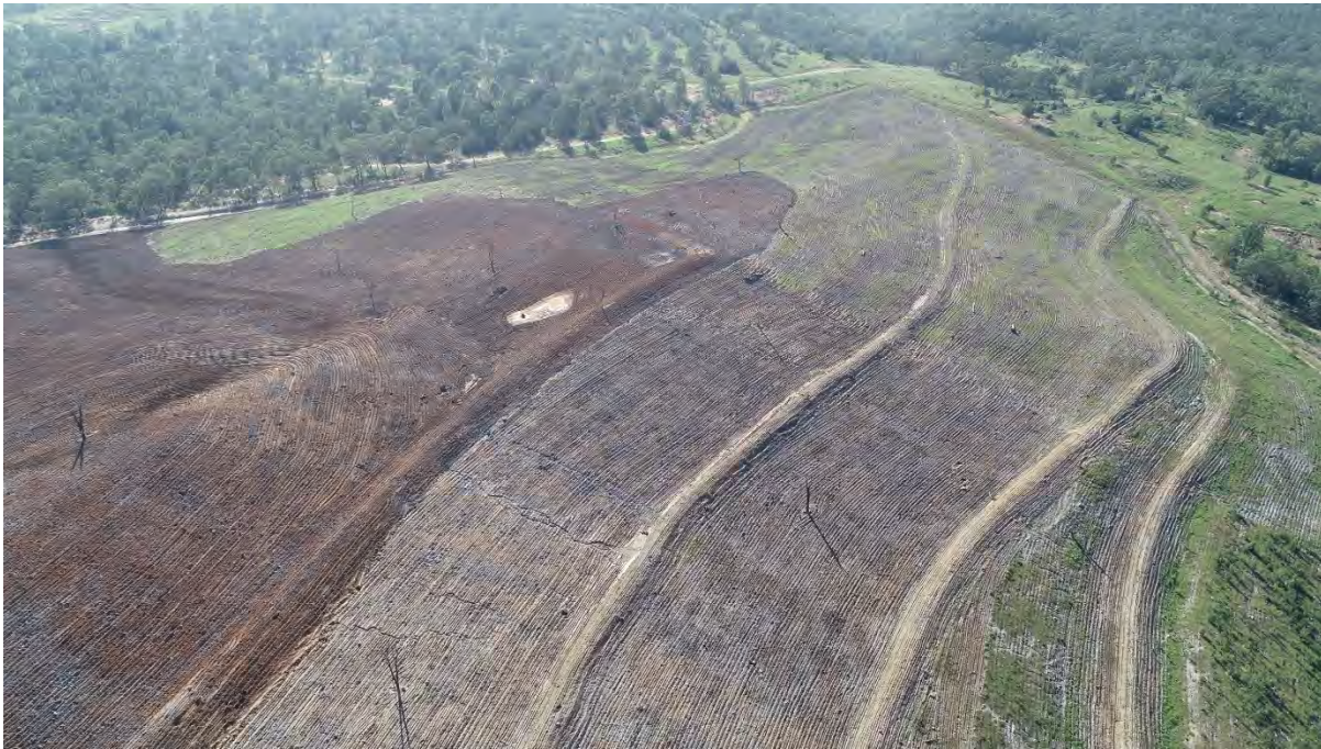
Photo 5 Example of traditional rehabilitation practices with contour banks (shaped in 2019 - right) next to natural landform design (shaped in 2020 - left).
