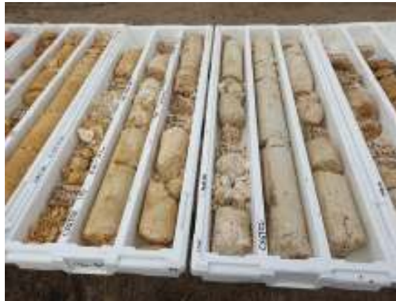
Selected Diamond Core Samples (PQ) from Geotechnical Hole CXGT02
