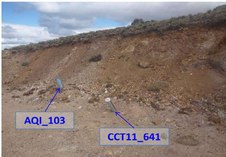
Figure 12-4 Vein 49 – Location Check of Twinned Drill Hole Locations (Cube site visit, 17/02/2017)
