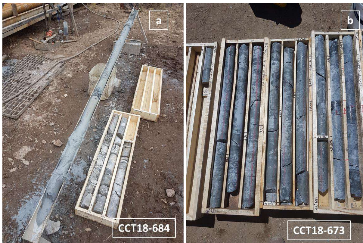
Figure 10-6: 2018 Drilling - HQ Core Extraction from Inner Tube (a); Core Cleaned and Laid Out in Wooden Core Trays (b) (Cube Site Visit, March 2019)
