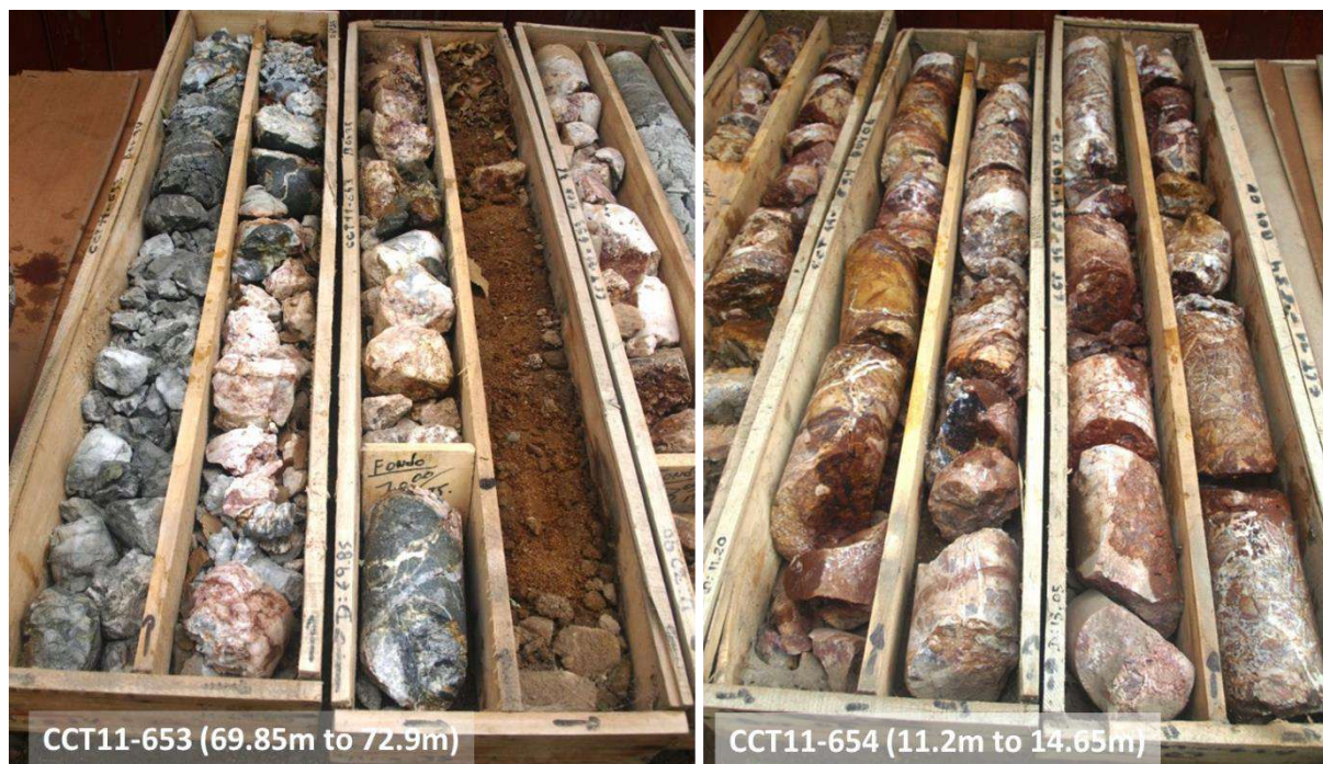
Figure 10-10: Examples of Core Recovery from Vein 49 PQ DD Core Drilled by PAS (Cube site visit, 17/02/2017)
