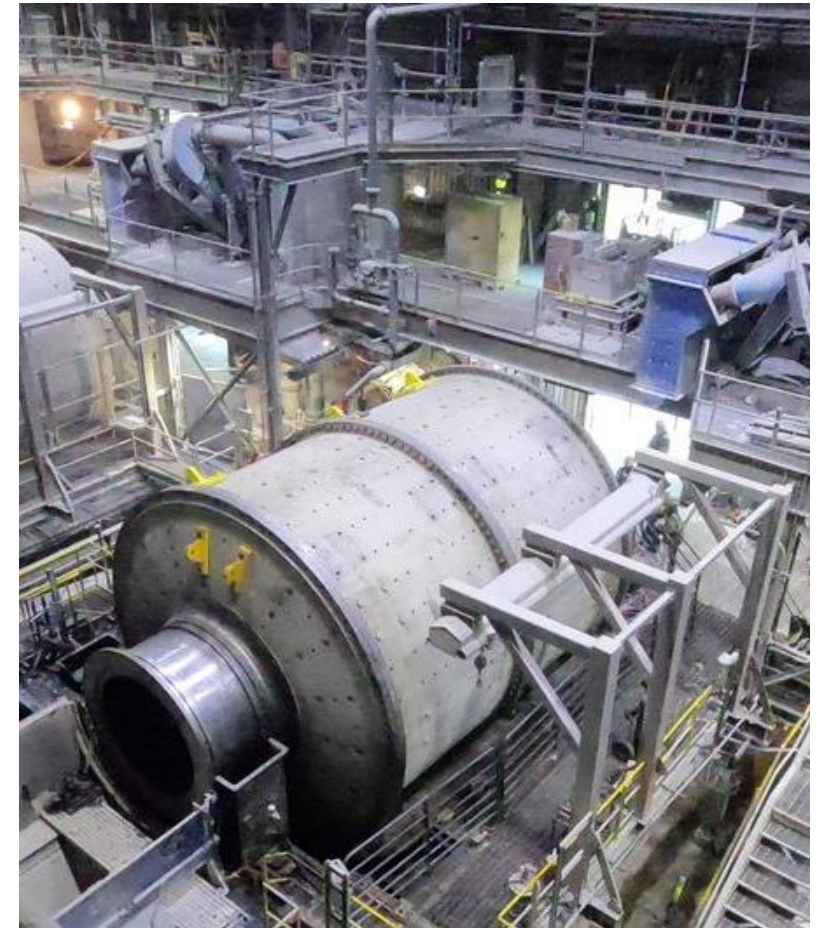
Ball Mill #3 installed safely in 30% less time than Ball Mill #4 last year.
