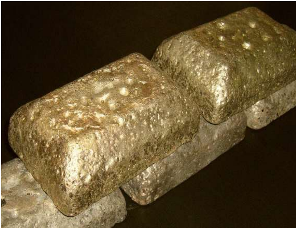
Figure 38. The final product – unrefined gold doré bars at the Company's Charters Towers project containing mainly gold and silver with ~5% impurities.
