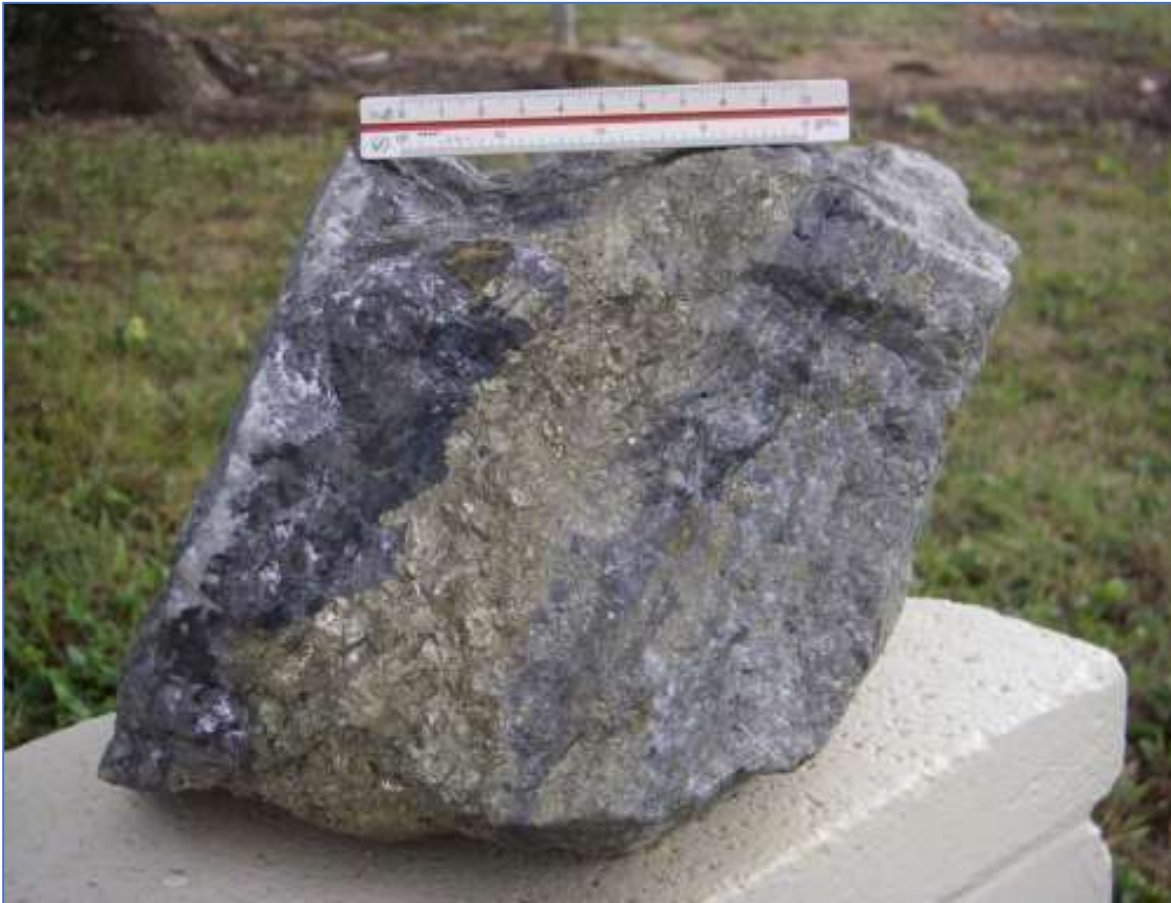
Figure 14 Typical high-grade gold ore, comprising pyrite (iron sulphide, brass coloured), galena (lead sulphide, silvery grey) and sphalerite (zinc sulphide, dark grey) in quartz and crushed granodiorite (“Formation”). The gold is too fine-grained to be visible. The top scale is in centimetres.
