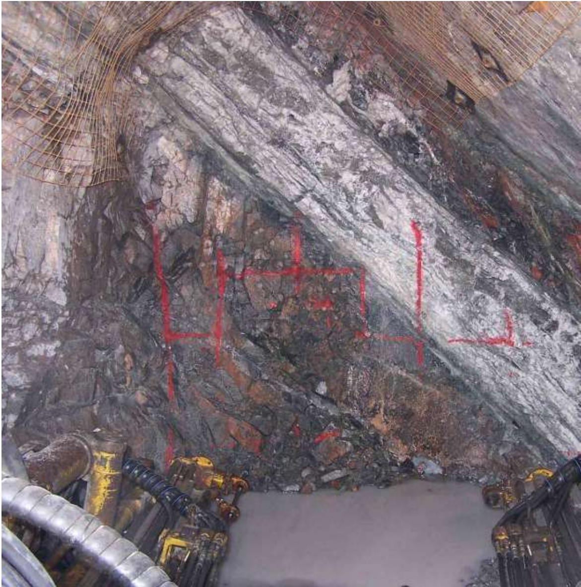
Figure 76. Gold-bearing quartz reef exposed in the Imperial Mine, prior to stoping (looking westerly).
