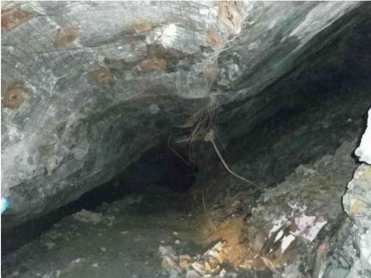
Figure 78. View looking east along the Sons of Freedom ore body in the Imperial Mine, showing the floor of the level drive, and the stope voids above and below the level. The ore has been cleanly extracted, with little dilution from the stable stope walls. While the access drive has to be about 3.5m x 3.5m to get drilling machines into the area, the stope slots between the levels are confined to the ore itself, minimizing dilution by maintaining a narrow stoping slot width.
