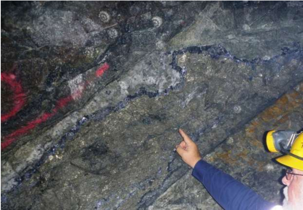
Figure 68. Where the ore body width is less than one metre, the grade is diluted out to an arbitrary width of one metre, as one metre is the minimum width that is likely to be mineable (looking easterly).
