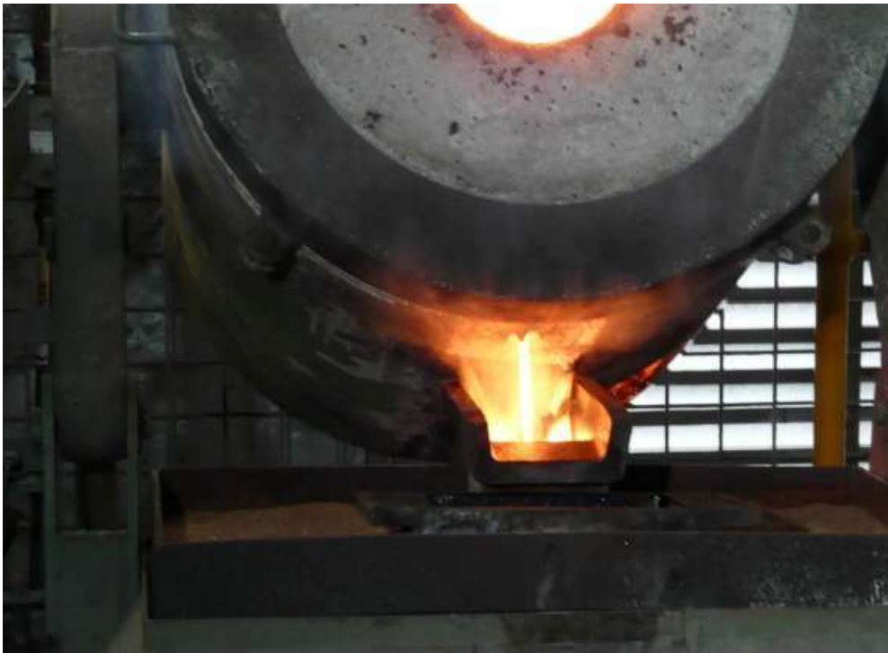
Figure 37. Pouring the gold doré bars after extraction and smelting at the Company's Charters Towers project.
