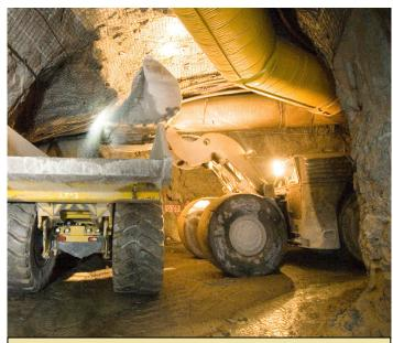
ABOVE: Underground during test mining loading rock into truck for haulage to the surface. This was at the 'Warrior' mine, located about 5 kilometres from 'Central'. Future mining will be at 'Central' where there are many more reefs.
