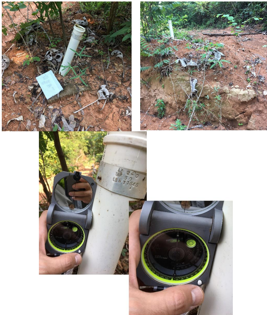
Figure 12-1: Collar Survey and Dip/Azimuth Measurement COR0001
