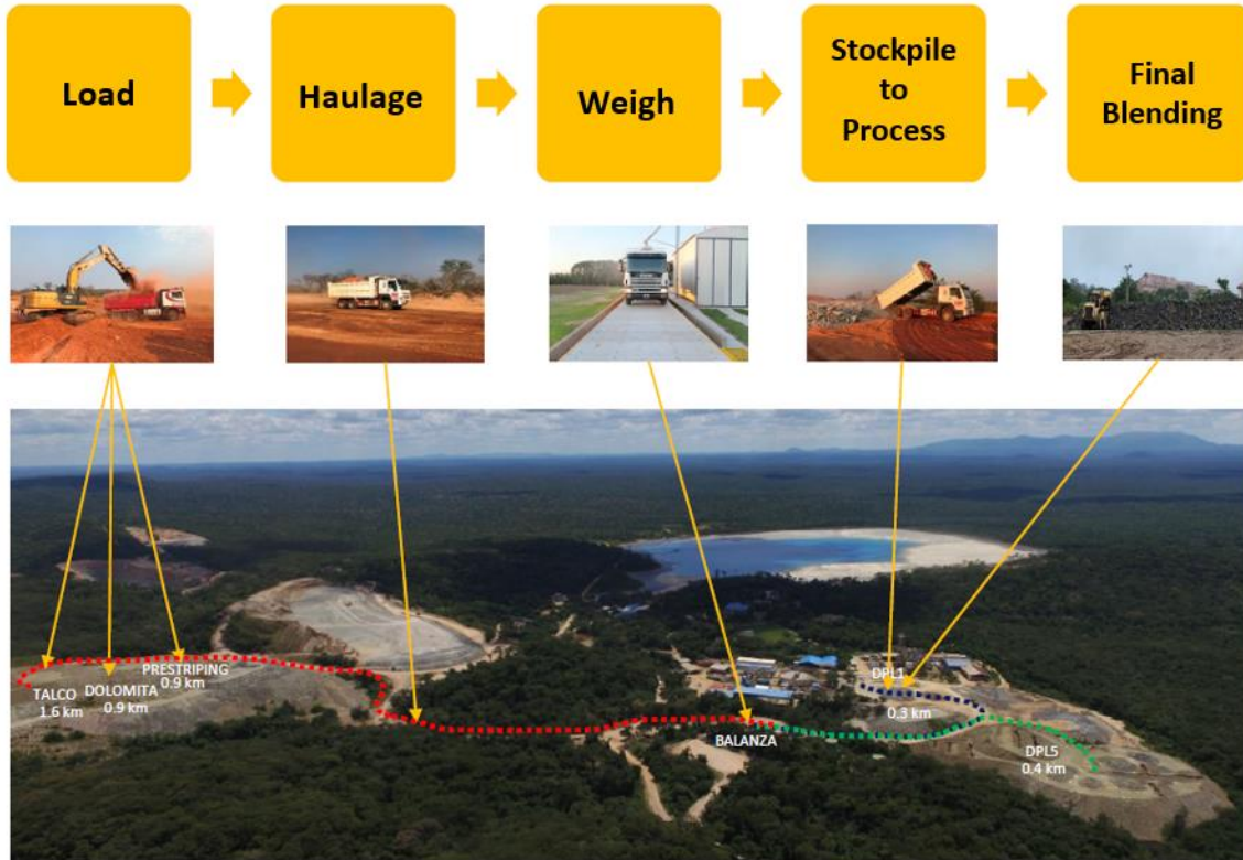
Figure 14. 1: Proposed flowsheet for Haulage
