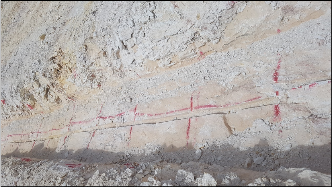
Figure 10.3: Typical Trench Sampling at Martinetas
