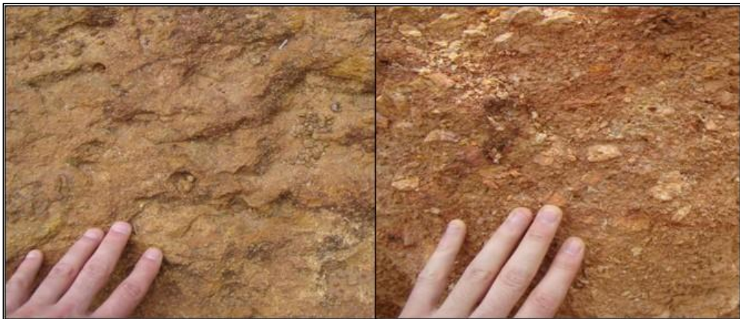
Figure 7.7: Sandy indurated mottled zone (left) and gravelly level showing fragments of mineralised quartz veins (right)
