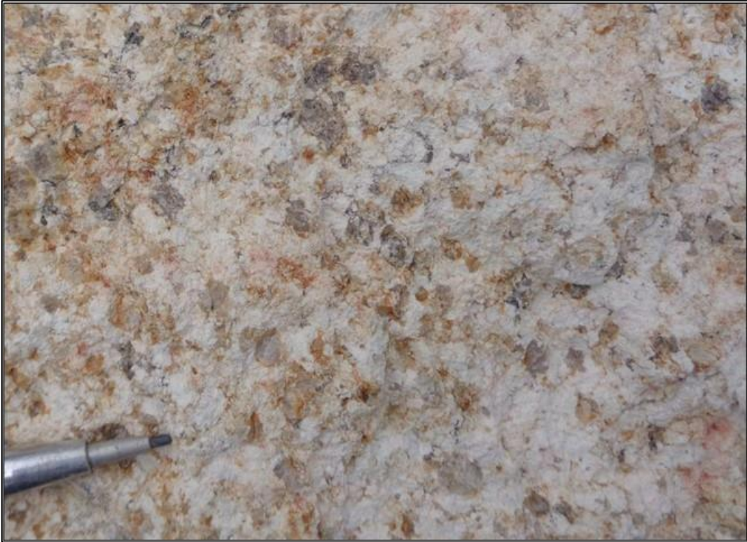
Figure 7.8: Upper saprolite (where the original fabric is partially preserved)
