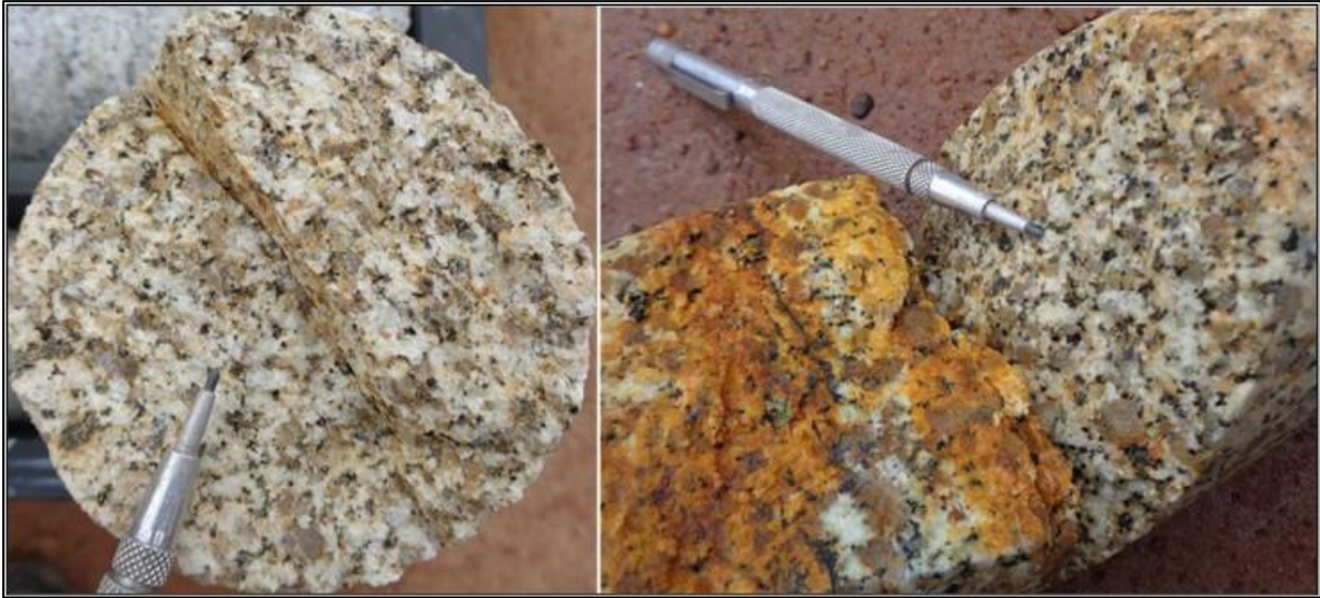
Figure 7.10: Transition zone between lower saprolite and fresh rock
