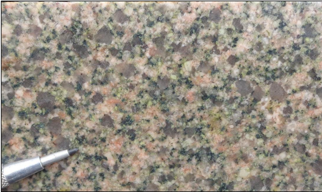
Figure 7.12: Distal epidote-chlorite-weak hematite alteration on granodiotite
