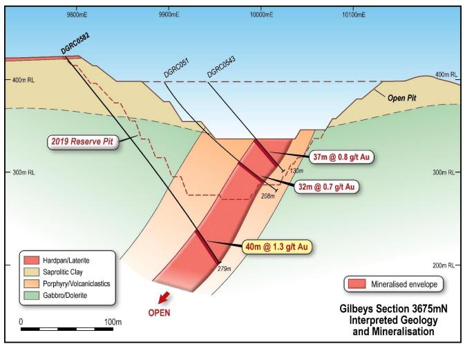
Figure 5: Gilbey's cross section 3675N showing recent RC drill hole DGRC0582
