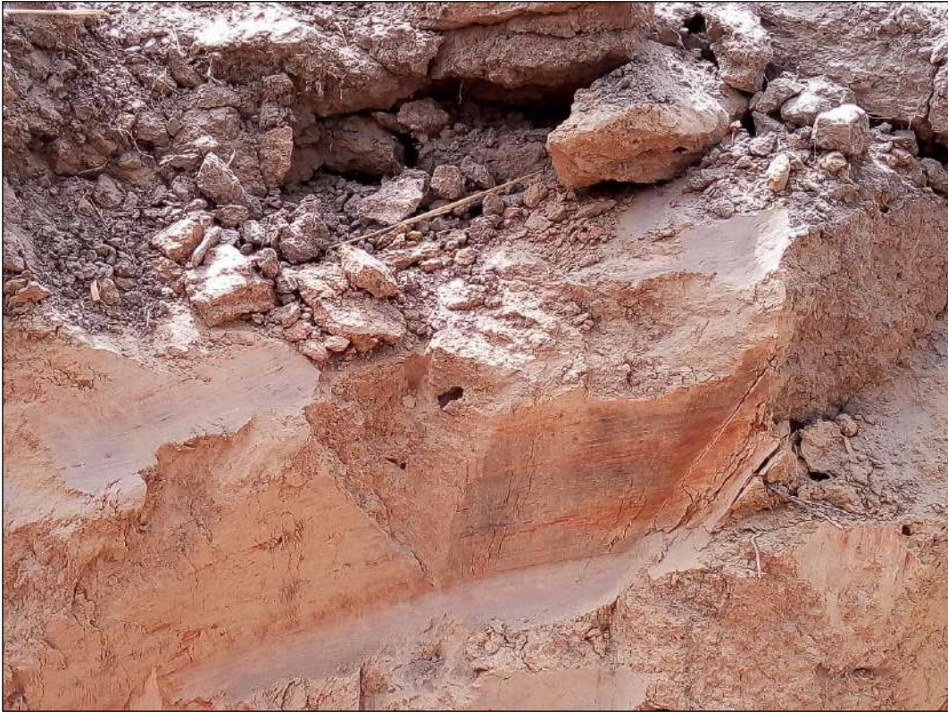
Figure 18.14: Close-Up of the Clayey Silt Near the Ground Surface Below Topsoil
