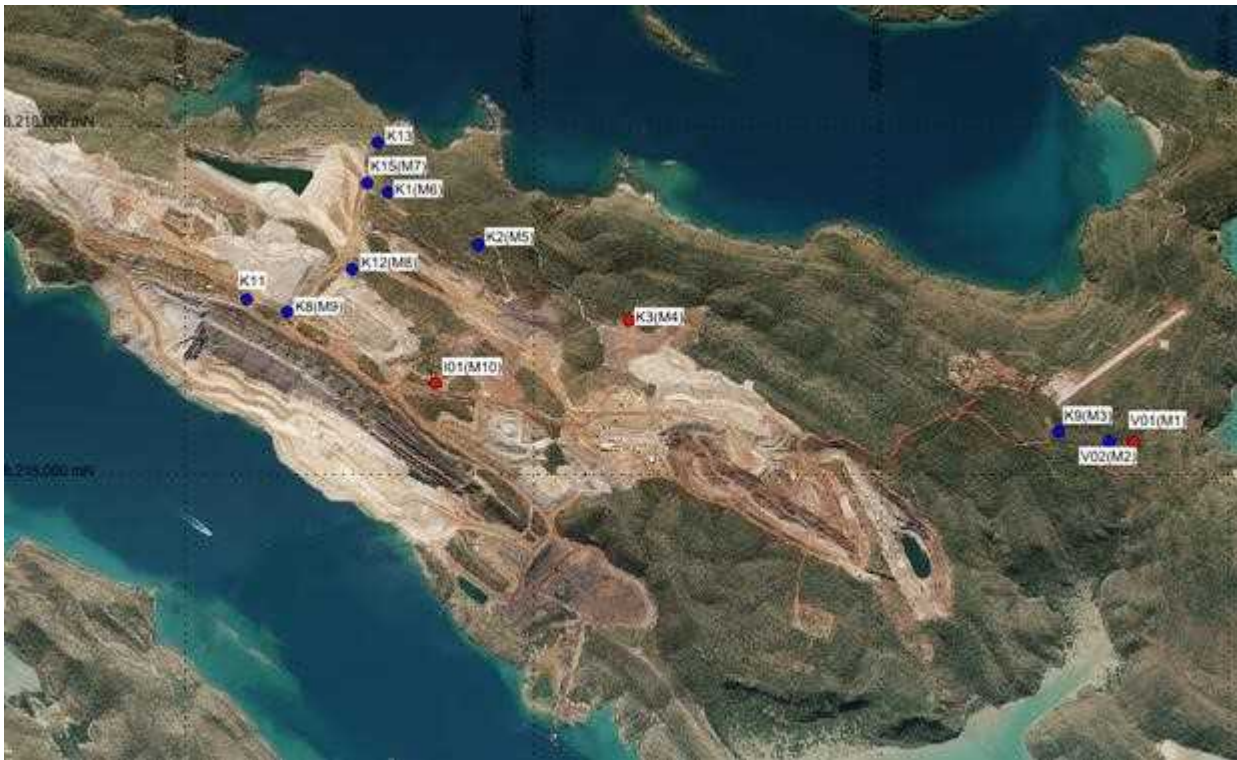
Figure 7-5: Location of Production Bores (red) and Monitoring Bores (blue).
