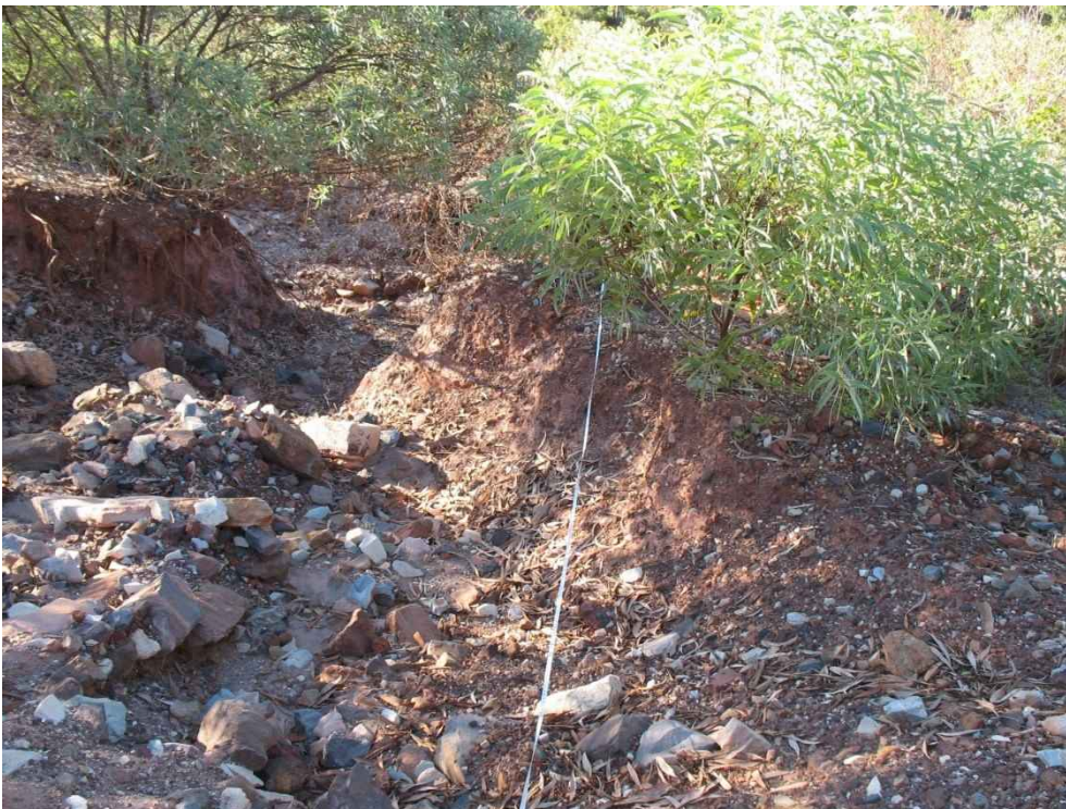
Plate 7-4: Erosion Gully at the Top of the WD4 LFA2 Transect – Poor Performance
