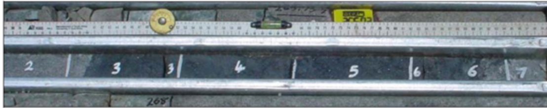
Figure 12.1: The top and bottom UG2 contact samples showing the inclusion of 2 cm of hangingwall and footwall respectively.
