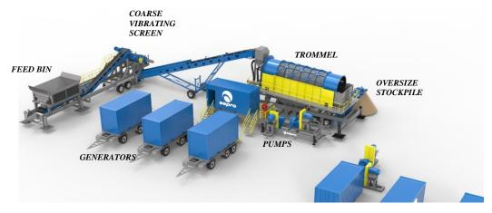
Figure 4 Lucky Bay Garnet Mine Mining Unit Plant
