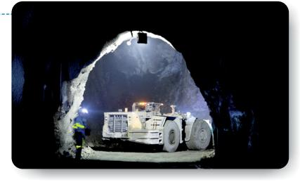
MATSA has implemented a tele-remote control system for underground equipment in Magdalena. This system allows the control of the loaders to excavate the stopes and equipment through a tele-remote control using video cameras and remote control from a cabin located at the surface. This innovation improves the safety and comfort of our employees. In the future the objective is to implement this system at the Sotiel and Aguas Teñidas mines.
