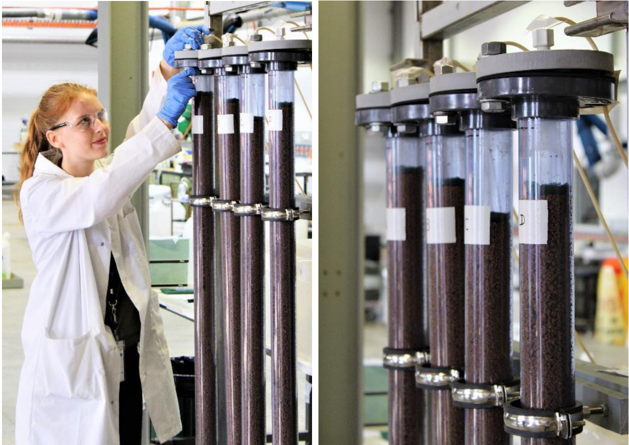
Figure 20: Heap leach columns under desorption (irrigation) at ANSTO Minerals in Sydney.
