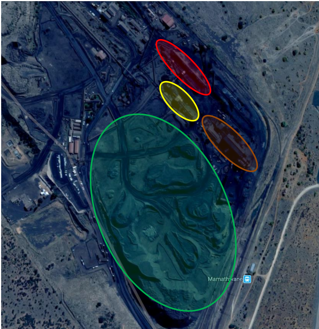
Figure 5.2-6 Higher magnification Google Maps satellite picture of Mamathwan Plant (red, yellow and brown ovals – OPP, DMS Sinter respectively), product and waste stockpile (green oval) area.
