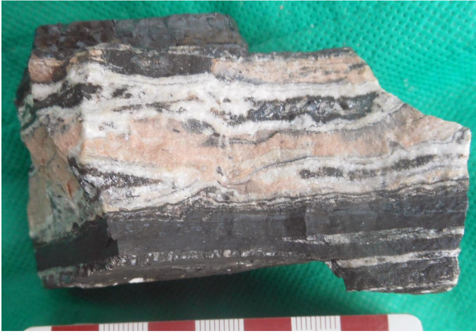
Figure 2.2-9 Sample from the Mamatwan ROM stockpile with high mineral composition variability (with permission: Gerry Ray)
