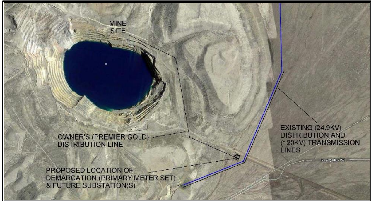
Figure 18-7 Electrical Site Plan
