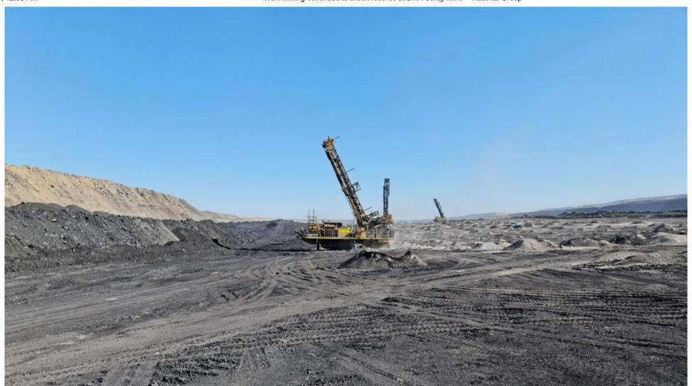
November drilling at BMA Saraji has been undertaken in 270mm holes ranging in depth from 30m to 65+m in tertiary material.
