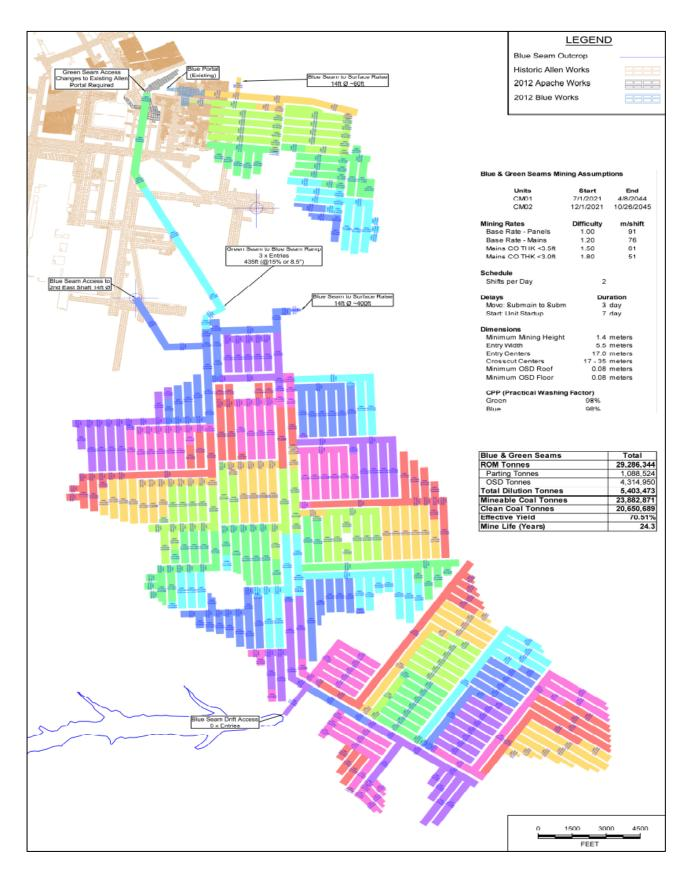
The Mine Plan was designed with a minimum coal seam height of 4.0 foot allowing for 6 inches of unavoidable out-of-seam dilution. Therefore, a mining height of 4.5 foot provides ample room for conventional lower profile underground mining equipment to operate remaining in the coal seam, and for the Mine to be adequately ventilated. Limiting coal recovery to 4.0 foot does reduce the recovery of some coal, but the
