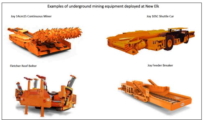
Image: examples of the main items of equipment in a room and pillar operation
