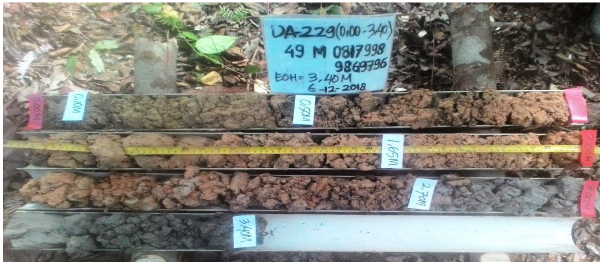
Figure 3-6 Core from auger hole DA-229 laid out for logging
