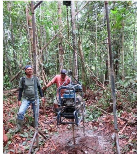
Figure 3-4 Mechanical auger drill used during phase 2
