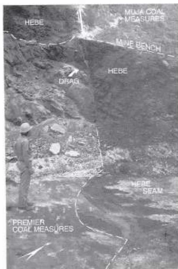
Figure 20. Tectonic structures exposed adjacent to Muja Fault, north highwall Muja Opencut. Windowed area is enlarged as Figure 21
