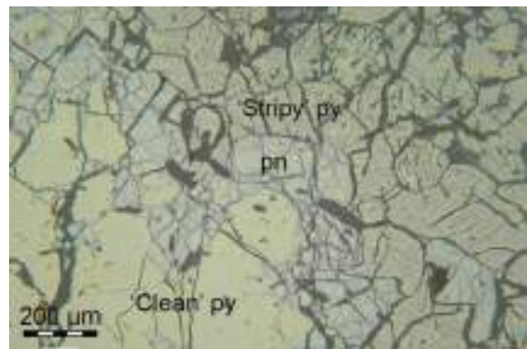
Figure 4.6h - M8049 734.49 – 'Clean' orbicular pyrite with altered pentlandite at its edge and then 'stripy' pyrite
