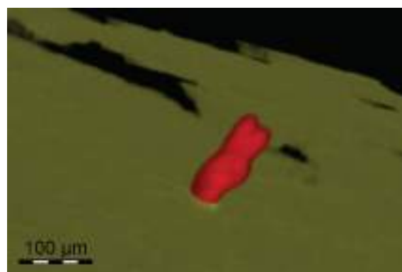
Figure 5.8d – HRXCT image showing a rod shaped grain that would equate to a round cross section in two dimensions.
