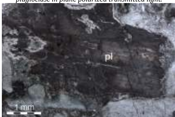
Figure 3.15e - Large plagioclase lath with alteration phases. Note the black colour in plane-polarised transmitted light.
