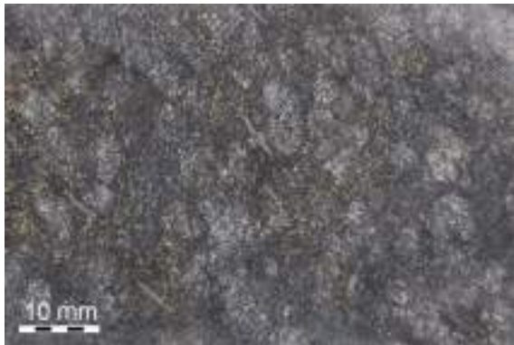
Figure 3.17a – 864.22 m sample has oikocrystic pyroxene and interstitial mineralisation.
