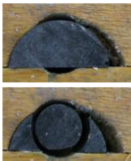
Figure 5.1 – subsampling of NQTK drill core (50.6 mm diameter) with a 20 mm diameter drill to produce cylinders for HRXCT scanning.
