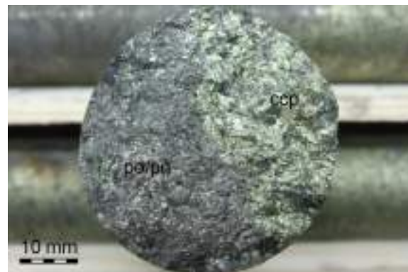
Figure 4.4d - massive sulphides showing segregation of pyrrhotite-pentlandite and chalcopyrite.
