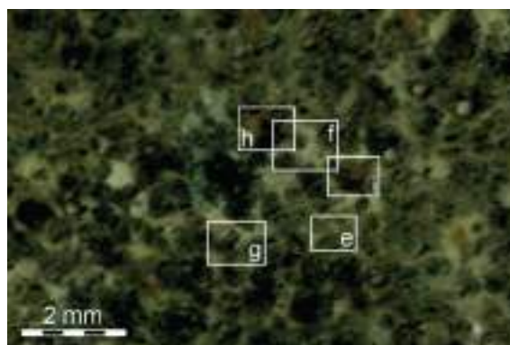
Figure 3.13b – Ti-rich pargasite can be separately identified from normal pargasite due to a reddish brown colour compared to normally colourless pargasite.
